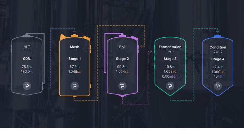
Image: Brewing process stages from heating and mashing to boiling, fermentation, and conditioning.
